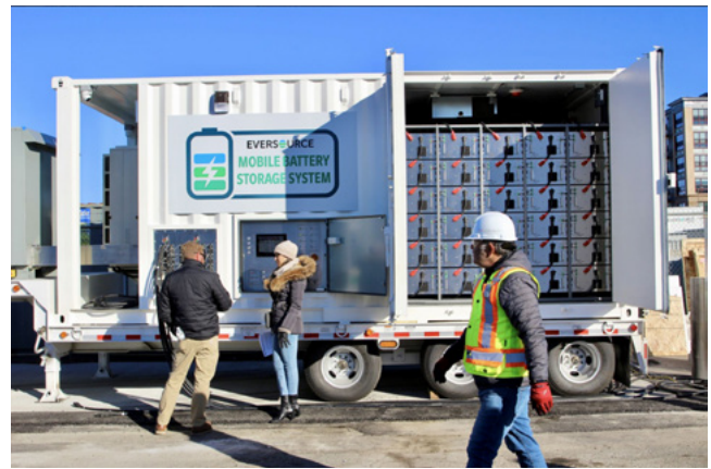
(b) Eversource’s 500MW, 2-Hour MESS Used During Outages
