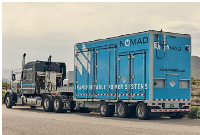
(a) Nomad Power’s Pilot of 1MW, 2-hour MESS
