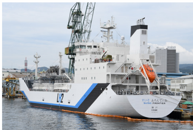
FIGURE 1: SUISSO FRONTIER, THE FIRST HYDROGEN GAS CONTAINER SHIP, IS CURRENTLY IN SEA TRIALS.
