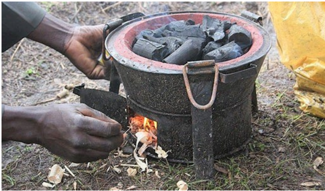
Two-thirds of Kenyan households still use a traditional stove as their primary cooking technology. Displayed here is the Kenyan ceramic jiko (KCJ), a mid-tier charcoal cookstove.
