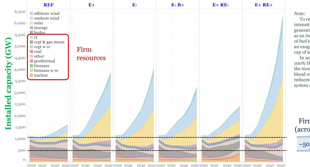
To reduce the carbon intensity of CCGT and CT generation,  $H_2$  is blended as an increasing fraction of fuel to these units, up to an exogenously specified cap of 60% (HHV basis). In sensitivities with
