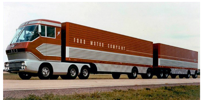
Figure 2: For decades truck manufacturers have shown that super-efficient trucks, like this gas turbine truck, are possible. Ford Motor Company's "Big Red" was built in 1964 (USDOE 2016).
