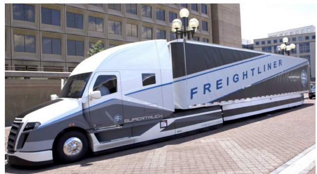
Figure 3: This DOE Super Truck from 2016 gets 12.2 mpg compared to an average fuel economy for tractor-trailers of just 5.8 mpg (USDOE 2016).
