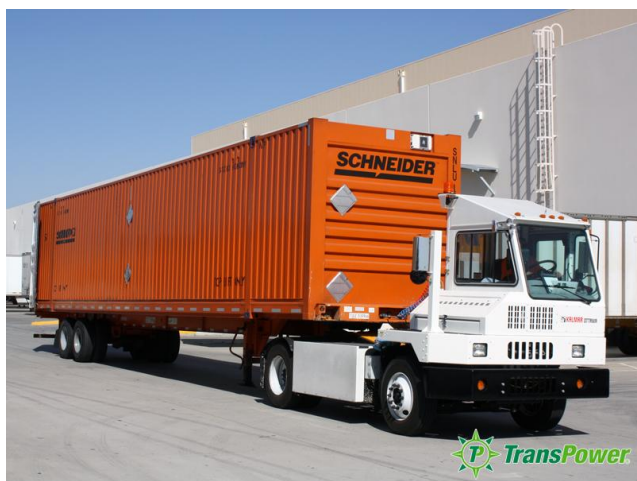
Figure 6: What a Super Efficient Urban Truck Might Look Like. This all-electric demonstration tractor has been operating at an IKEA Facility in California since 2014 (TransPower).
